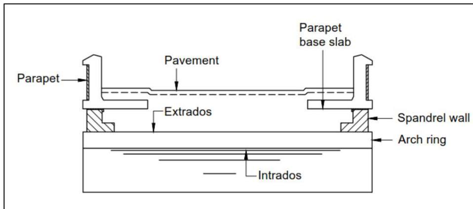
**Figure 4-1: Reconstruct parapet on a masonry arch bridge (CD376 Unreinforced Masonry Arch Bridges)**
