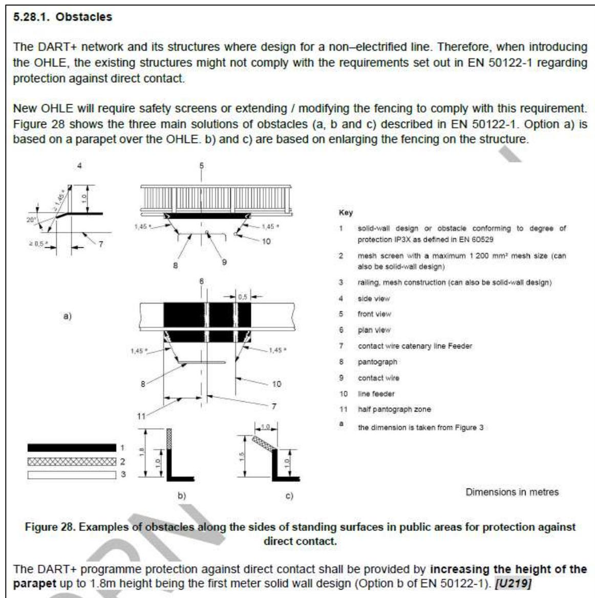
Based on the requirements of this document, a 1.8m parapet height conforming to Option (b) is required to provide protection against direct contact with the overhead wires.
